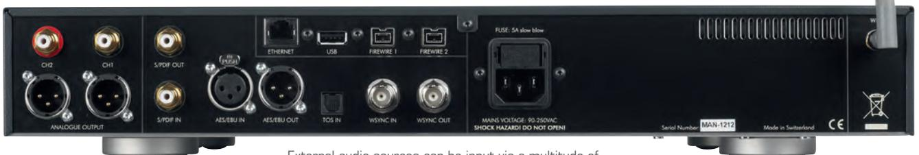
External audio sources can be input via a multitude of connectors. Even external clocks are accepted.
